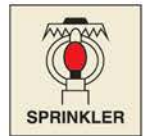
Space protected by sprinkler
