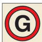
Emergency source of electrical power (generator)
