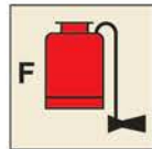
Portable foam applicator
