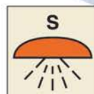
Space protected by sprinkler system
