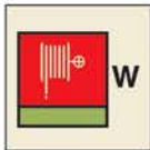
Water fire hose & nozzle
