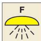
Space protected by fixed foam fire extinguishing system
