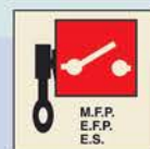
Remote controlled fire pumps or em. switches 6020 EE, GG & JJ
