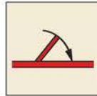
'A' Class self-closing fire door
