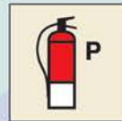
Powder fire extinguisher
