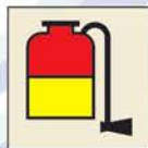
Portable foam applicator unit
