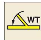
'B' Class self closing watertight fire door
